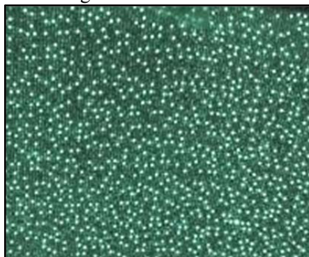
Fig. 2. Infrared dots projected by Kinect seen with a night vision camera.
